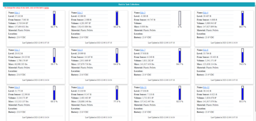
Figure 4: Tank collections view on ABM web-based portal showing inventory status of 12 silos.
